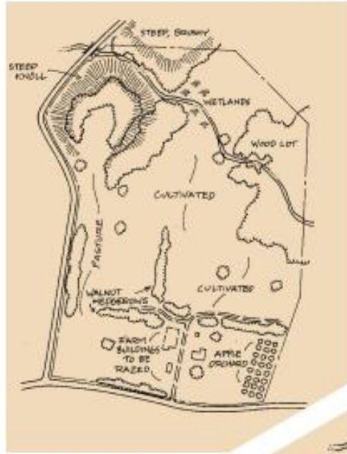
Figure 16. A natural resource inventory identifies all important natural characteristics of a site.
